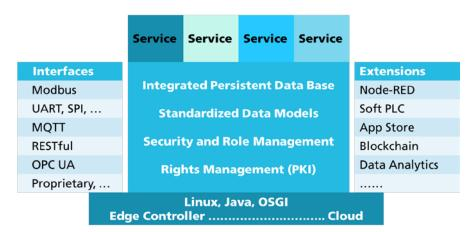
Around a core, the actual OGEMA platform, more and even complex interfaces and applications can be supplemented that can act together as needed.
