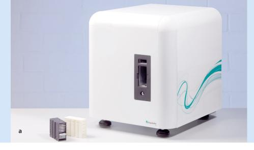
The detection system is based on the SCube® Scanning Plattform (a). First, an overview scan of the so-called thick smear in low magnification is acquired (b). After the overview scan a configurable number of fields will be scanned in high magnification in the center of the smear; an example field is shown in (c). In (d) detection results for possible parasites, *i.* e. plasmodia, are displayed. Detected plasmodia will be presented in a graphical user interface for manual review and approval.
