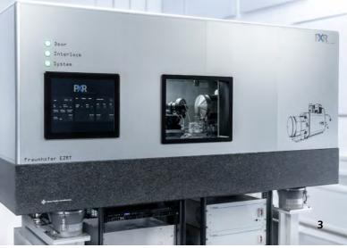
2 3D analysis with microscopic reand failure analysis on lithium electrodes for battery research with a voxel sampling of 140 nanometers.
