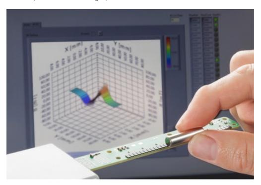
The line camera visualizes magnetic field values in real time. © Fraunhofer IIS/Max Etzold | Picture in color and printing quality <a href="https://www.iis.fraunhofer.de/en/pr">www.iis.fraunhofer.de/en/pr</a>.
