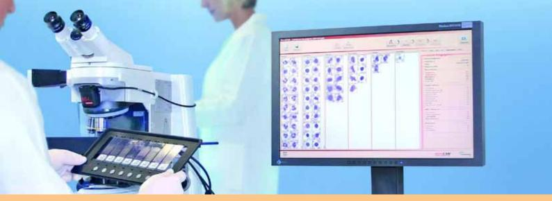
Figure 1: HemaCAM consists of a fully automated microscope with a connected camera, computer and graphical user interface and allows for automatically analyzing blood smears and supports the classification of the leukocytes
