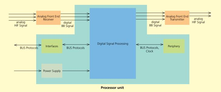
Figure: Block diagram of the on-board processor unit
