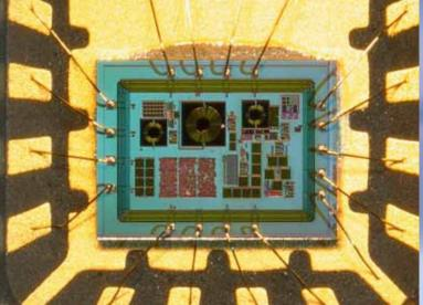
Figure 1: The 2.2 mm x 1.7 mm wake-up receiver chip contained in the QFN16 plastic case (5.0 mm x 5.0 mm)
