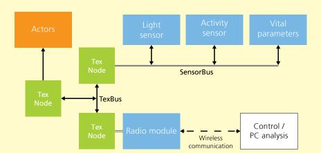
Figure 1: Textile-based network
