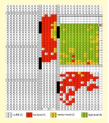
Figure 3: Reception card of a transmitter
