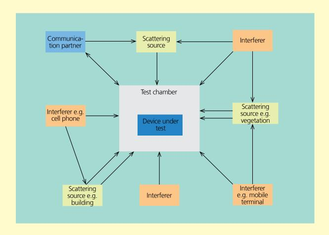
Figure: Diagram illustrating the OTA testing system
