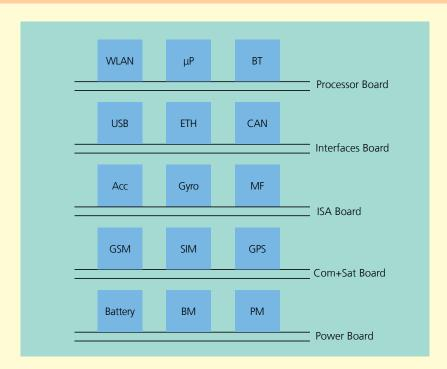
Figure 2: Concept for the modular miniLOK
