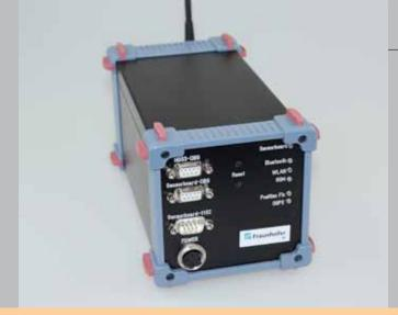
Figure 1: Development platform for seamless location by GNSS, WiFi and inertial sensors
