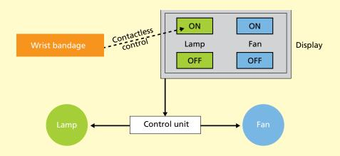
Figure 2: EASyCONTROL – contactless device control
