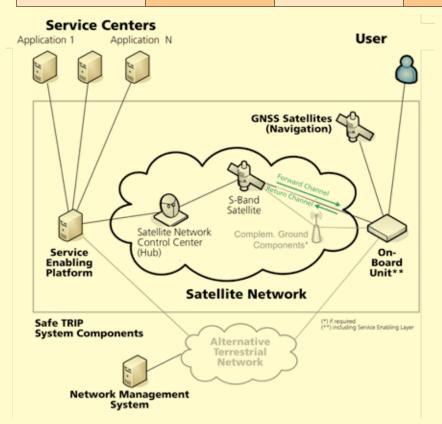
Figure 1: SafeTRIP system concept
