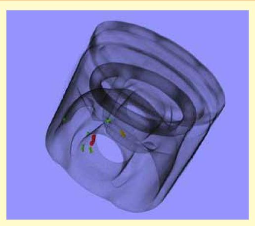
Figure 2: 3-D presentation of the computer tomography data record of a casting with marked surface defects
