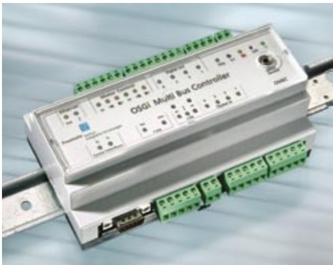
Bild 1: OSGi Multi-Bus-Controller Figure 1: OSGi Multi-Bus Controller
