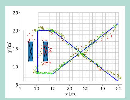
The test trajectories are in between the training trajectories, at different scales and both orthogonally and at an angle of 45°.
