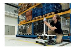
Testing with 5G UL-TDoA positioning, evaluated using an autonomous mobile robot.
