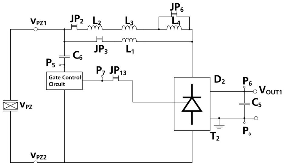
Fig. 3: SSHI AC-DC converter
