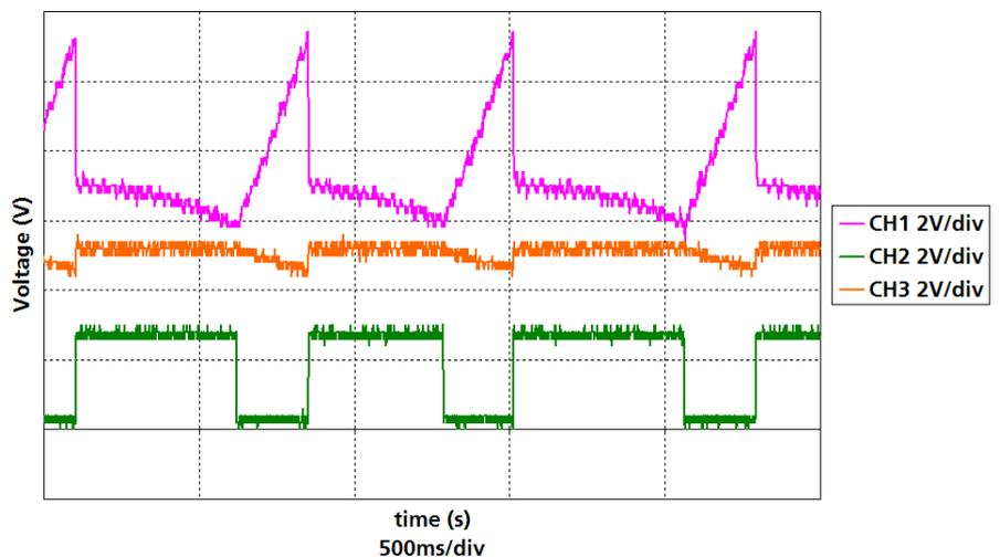
Fig. 7: Steady-state operation of the regulated output voltage on pins X3-1 and X3-2
