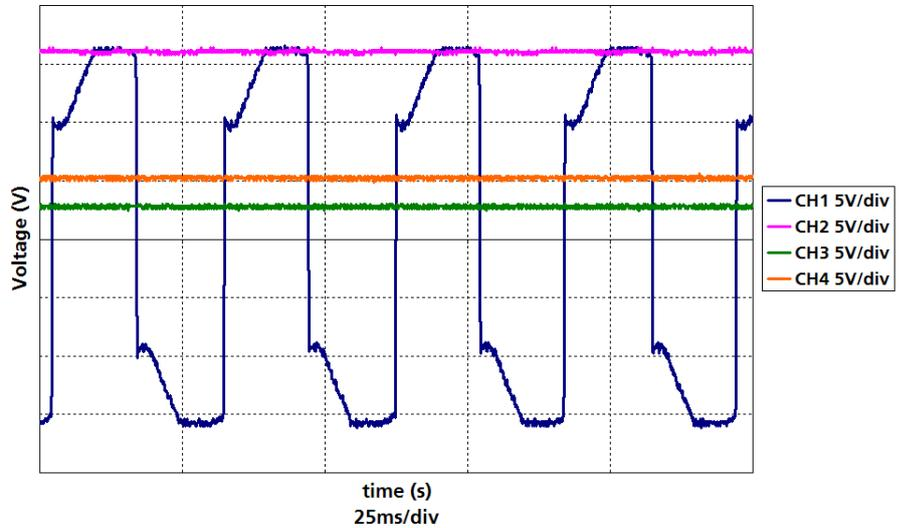
Fig. 6: Steady-state operation of the regulated output voltage on pins X3-1 and X3-2
