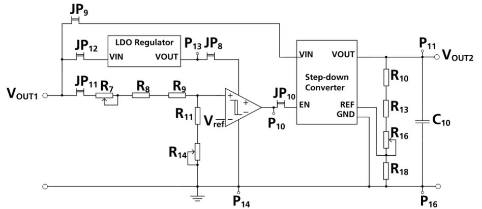
Fig. 4: Schematic for the DC regulated output voltage
