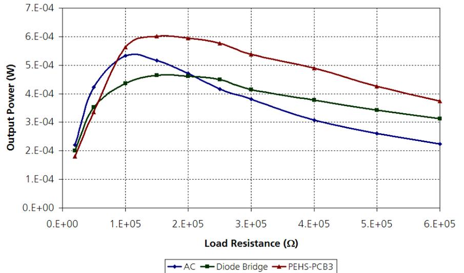
Fig. 2: Harvested power as a function of the load for different topologies employing a piezoelectric element at 16.7 Hz.
