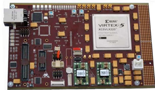
**Figure 8.** GNSS rapid-prototyping baseband receiver
