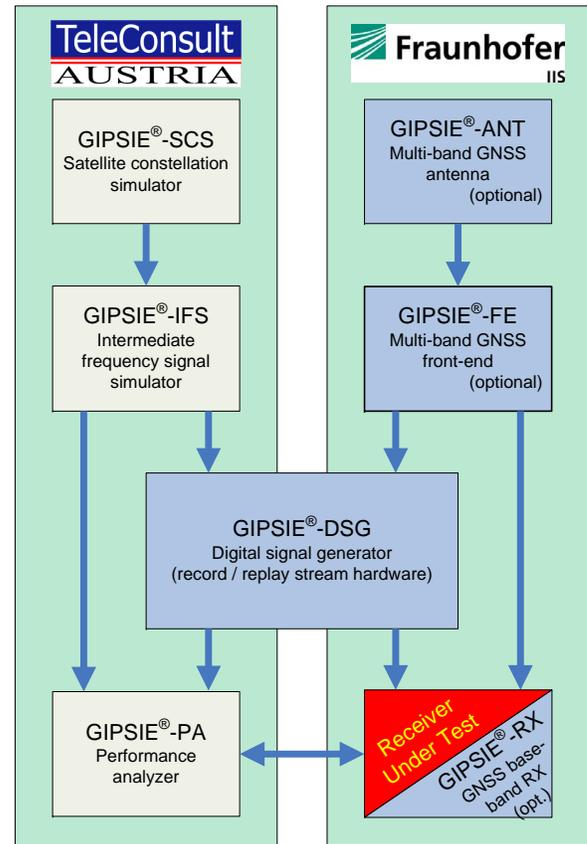
**Figure 9.** GIPSIE® system architecture
