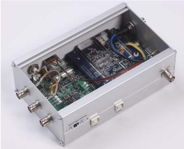
**Figure 7.** Portable RF front-end USB solution
