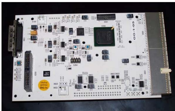
**Figure 5.** Digital signal generator and recorder interface adapter hardware
