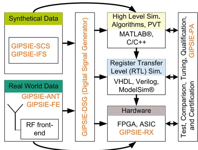
**Figure 13.** Using the GIPSIE<sup>®</sup> environment for GAMMA-A digital baseband development
