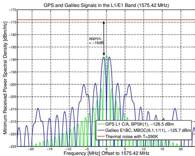
**Figure 1.** Negative signal-to-noise ratio of GPS and Galileo signals
