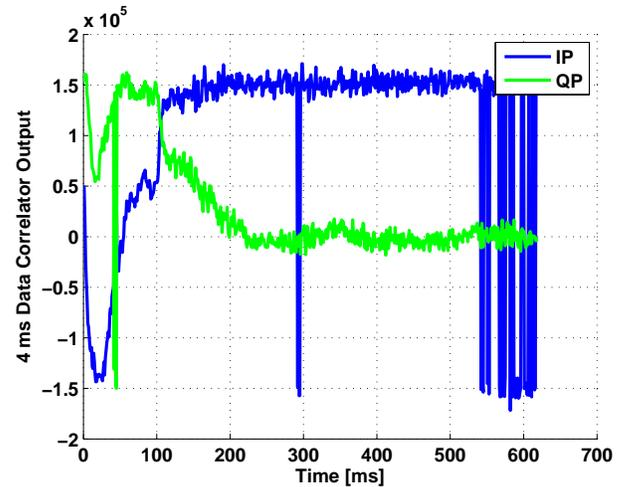
**Figure 12.** E1 data prompt correlator going into tracking with recorded data
