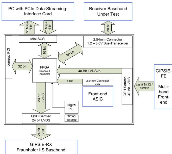
**Figure 4.** Digital signal generator and recorder interface adapter block diagram
