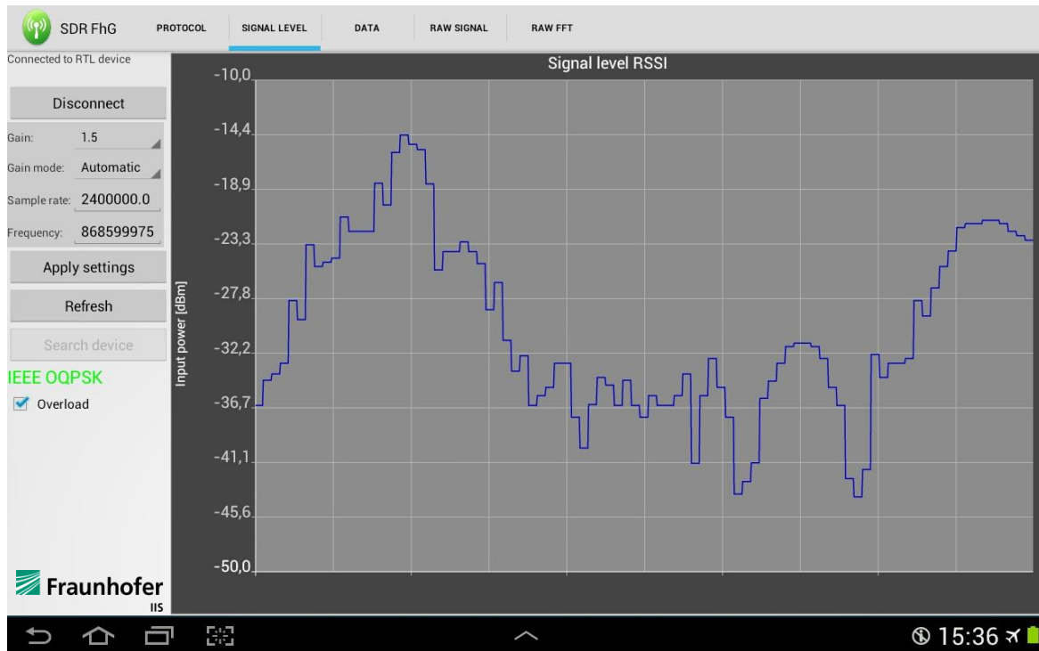
Figure 4 – Traffic Detective – History of signal strength
