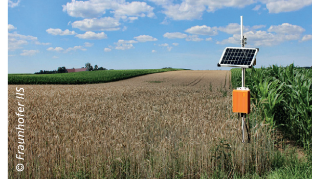
Energy self-sufficient mioty® base station for agricultural applications
