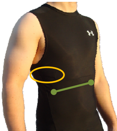
Figure 1: Applied FitnessSHIRT with integrated sensors (ECG – yellow, Respiration band – green)
