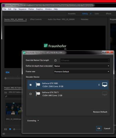
JPEG XS is a new codec for IP workflows in studio environments, for local video networks and for VR/AR applications which allows transferring high-resolution video data over standard Ethernet or other wired connections. The codec is a mezzanine compression codec which works with limited computing resources. The Fraunhofer IIS JPEG XS development can be used for lowest complexity and platform-independency applications at compression ratios from 2:1 to 10:1.
