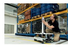
Testing with 5G UL-TDoA positioning, evaluated using an autonomous mobile robot.
