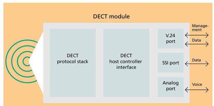
Our DECT solutions are specially geared towards industrial applications. Among their features are an extended operating temperature range, integrated antennas, patented antenna diversity technology and customer-specific software.
