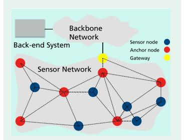
Reference model of a wireless sensor network
