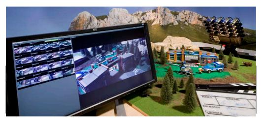
Capturing the light field: The new array from Fraunhofer includes 16 cameras (see it in picture's right above angle). So it is possible to rejust sharpness and camera angle even after the original recordings. © Fraunhofer IIS/Kurt Fuchs | Picture in color and print quality: www.iis.fraunhofer.de/pr.
