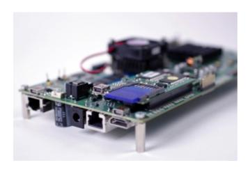
VEMPIRE® –Versatile embedded platform for image recognition. © Fraunhofer IIS/Bianca Möller | Image in color and printer quality: www.iis.fraunhofer.de/pr.
