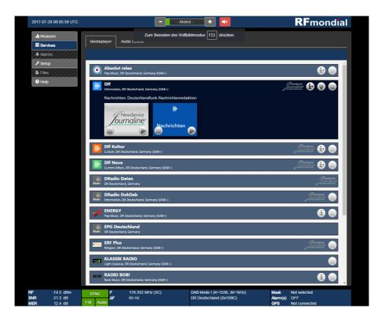
The Fraunhofer MultimediaPlayer technology is integrated in RFmondial's new RF-DAB monitoring receiver and enables the presentation of all DAB+ services. ©RFmondial | Picture in print quality: www.iis.fraunhofer.de/en/pr
