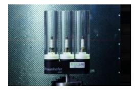
With PolyCT, measurement series can be tested up to three times faster The image shows the conversion kit loaded with three spark plugs. © xray-lab
