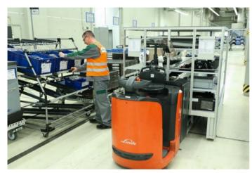
Pick-by-Local-Light being tested at Volkswagen: PbLL guides pickers through the order picking process and shows the required quantity on a display. © Volkswagen
