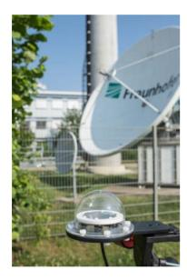
Using this C-band antenna (foreground), Fraunhofer IIS successfully transmitted sensor data via a geostationary satellite. © Fraunhofer IIS/Sabine Metzger | Picture in print quality: www.iis.fraunhofer.de/en/pr
