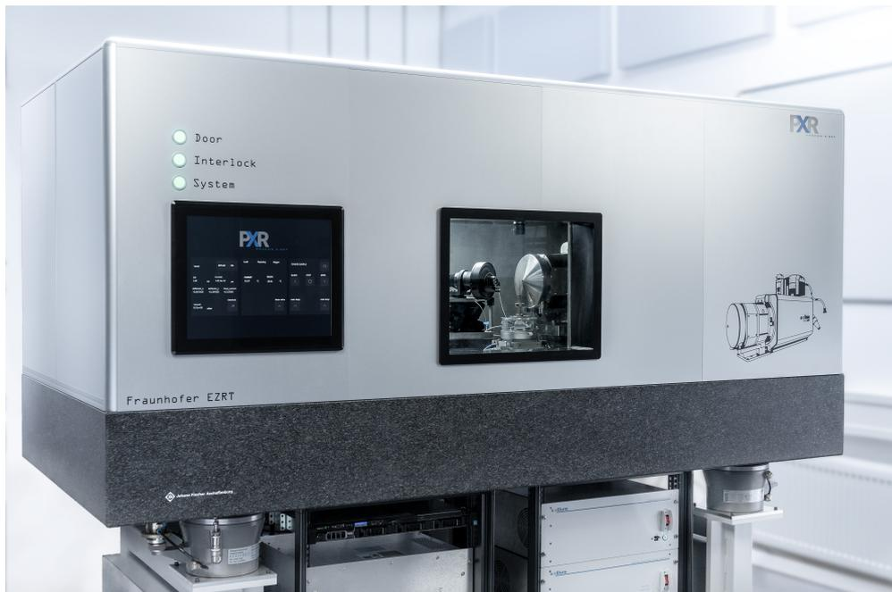
**Compact stand-alone design for easy integration into your lab environment. The "ntCT" system offers a unique solution for high-resolution measurements. By applying the latest developments in X-ray research, it is way ahead of established industrial micro-CT scanners. © Fraunhofer IIS**
